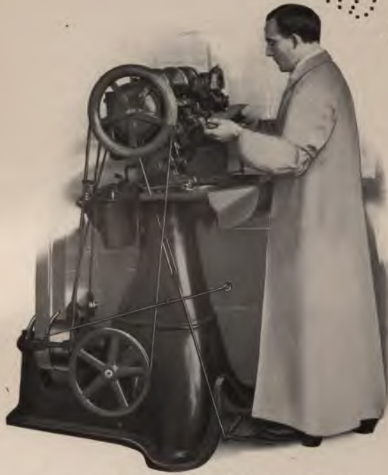
Operating the Goodyear Stitching Machine
